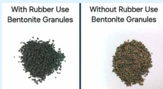
Bentonite granules produced with and without use of Rubber Field study at one of the Bentonite Units
