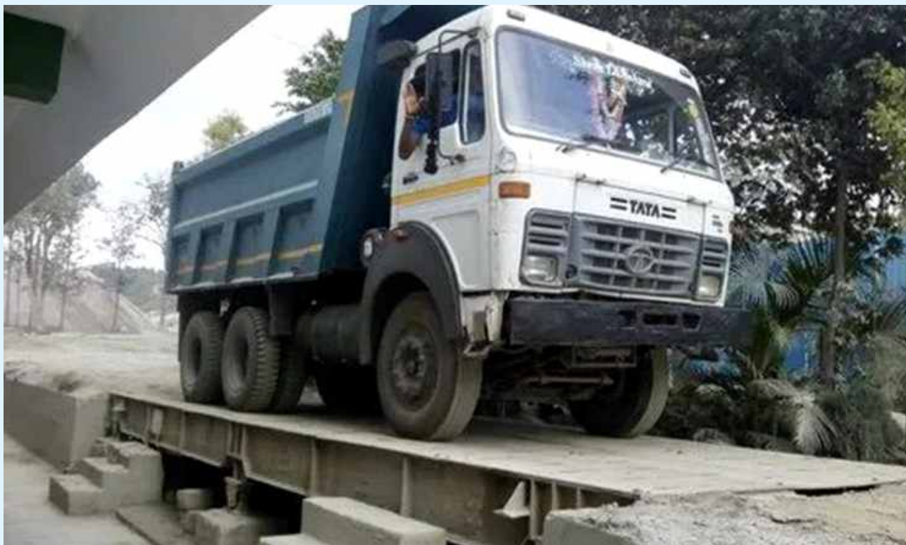
The weighment of coal laden Tippers on the weighbridge in the coal mines area
